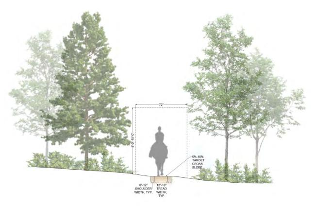
FIGURE 8.5: CLASS 2 EQUESTRIAN TRAIL ELEVATION
