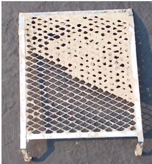
Painting grate during clean-up (DSCN0864.jpeg). Each grate has about 360 holes, which can be cleaned at the rate of about 7 seconds per hole.
