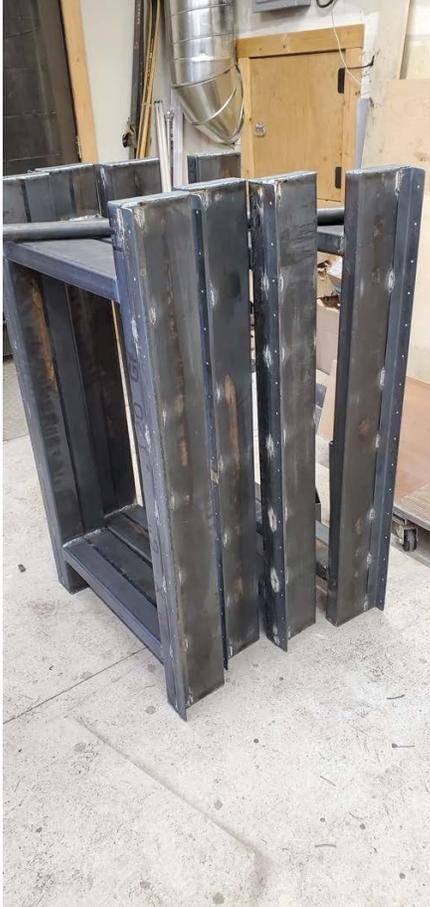
Left: Welded frames for carriage-mounted benches.
